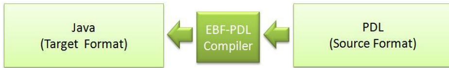
Figure 68: The EBF-PDL Compiler as a black box that maps the source format (PDL) into the target format (Java).
